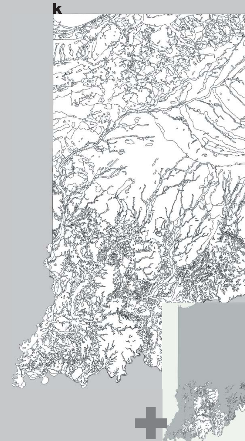
IGS Miscellaneous Map 49—Quaternary Geologic Map of Indiana by Henry H. Gray (1989)—displayed as vector contour lines. Areas designated as shallow bedrock were used as the upper layer in the final thickness of the unconsolidated deposits map (map l ).
