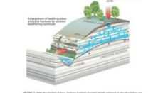
FIGURE 2. A karst basin with a sinkhole. The diagram shows the relationship between the karst features and the overlying glacial drift and alluvium.
