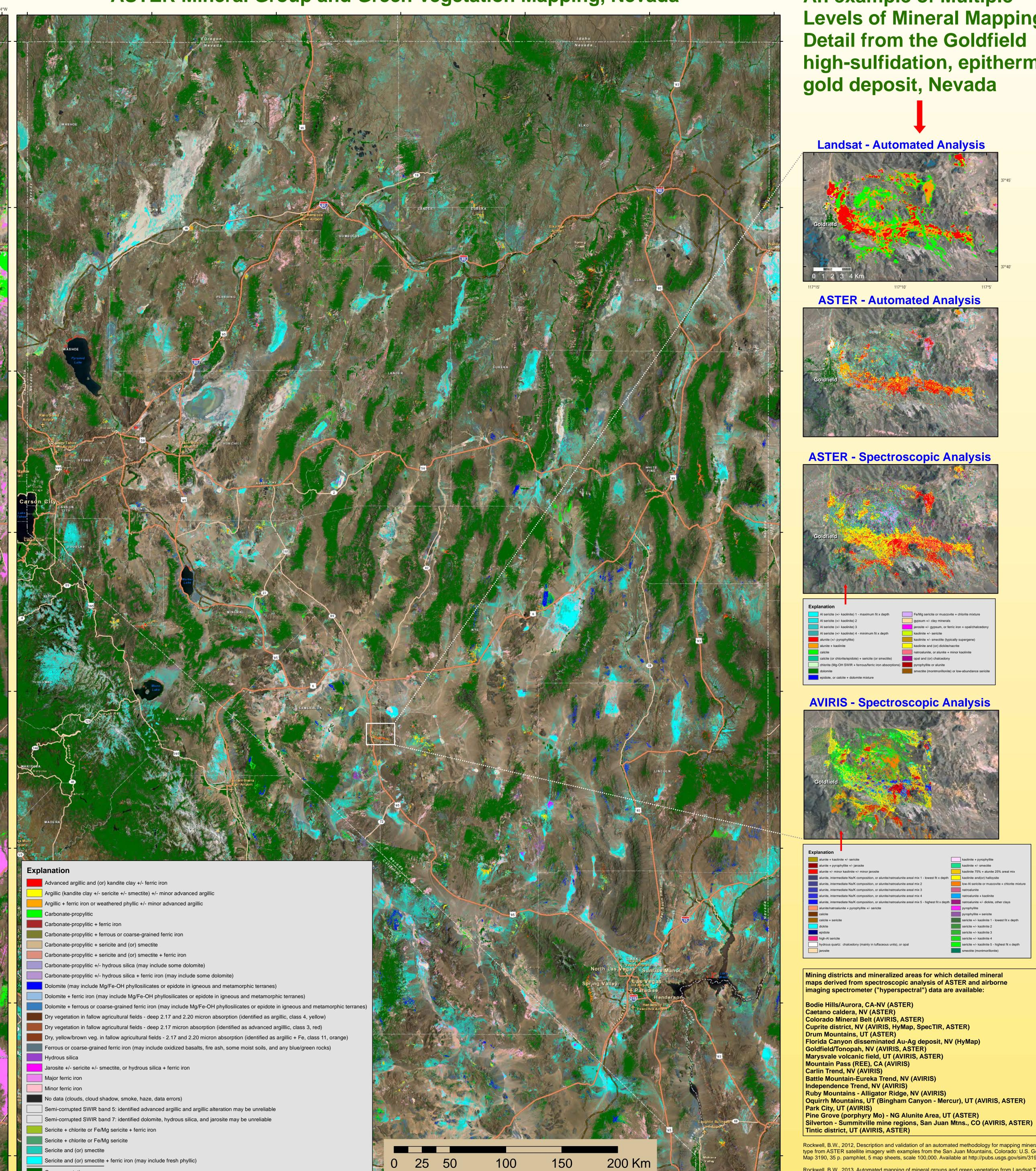
An example of Multiple **Levels of Mineral Mapping Detail from the Goldfield** high-sulfidation, epithermal gold deposit, Nevada
