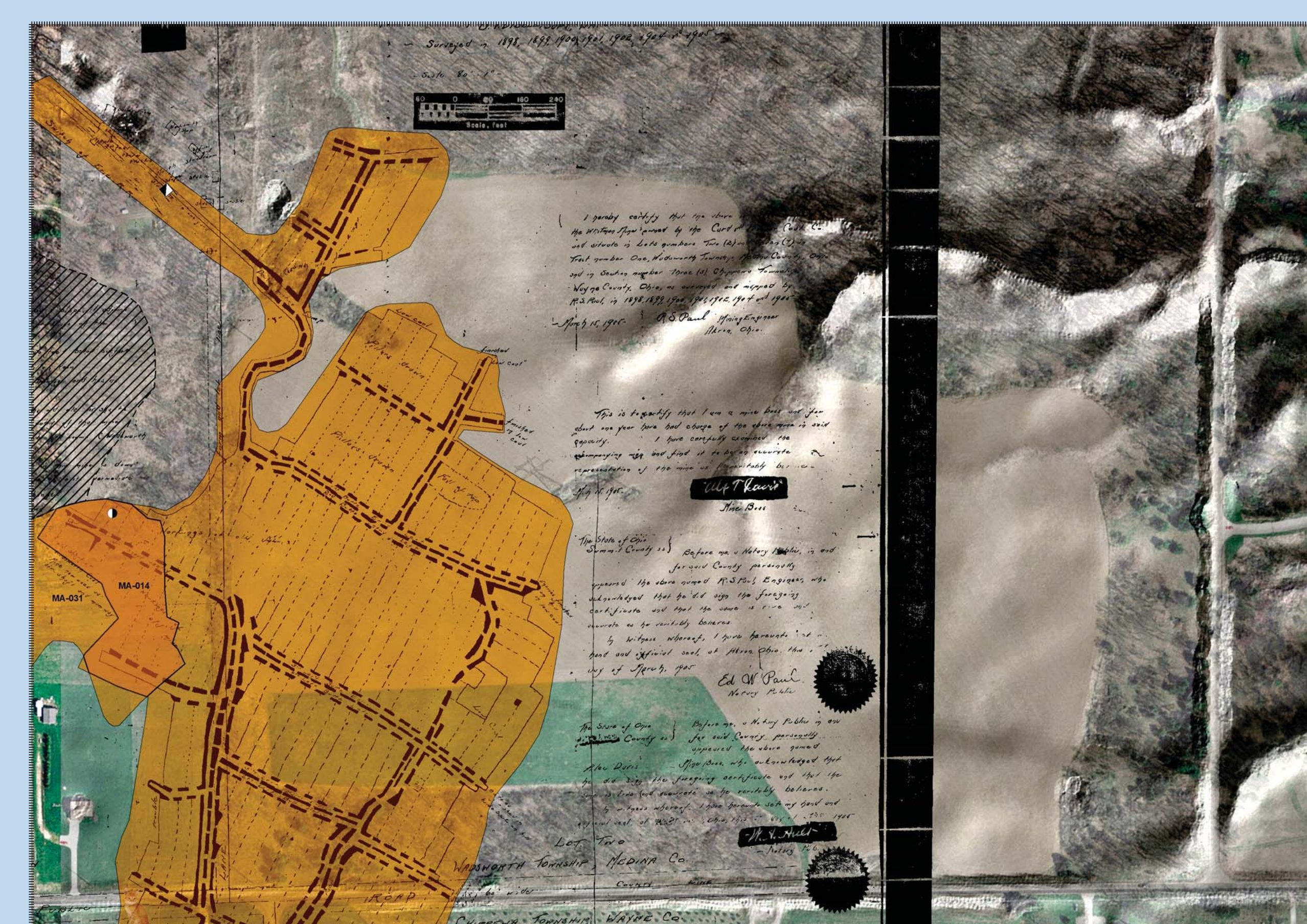
FIGURE 4b.—Overlay of the abandoned-mine map and the gridded LiDAR hill shade. The overlay clearly shows that the unusual pattern on the left side of the figure is due to slope entry to the mine. The other unusual patterns in the center of the figure may be caused by collapse of unmapped entries from an extension of the abandoned-underground mine. Further field work is necessary to confirm or refute this hypothesis.
