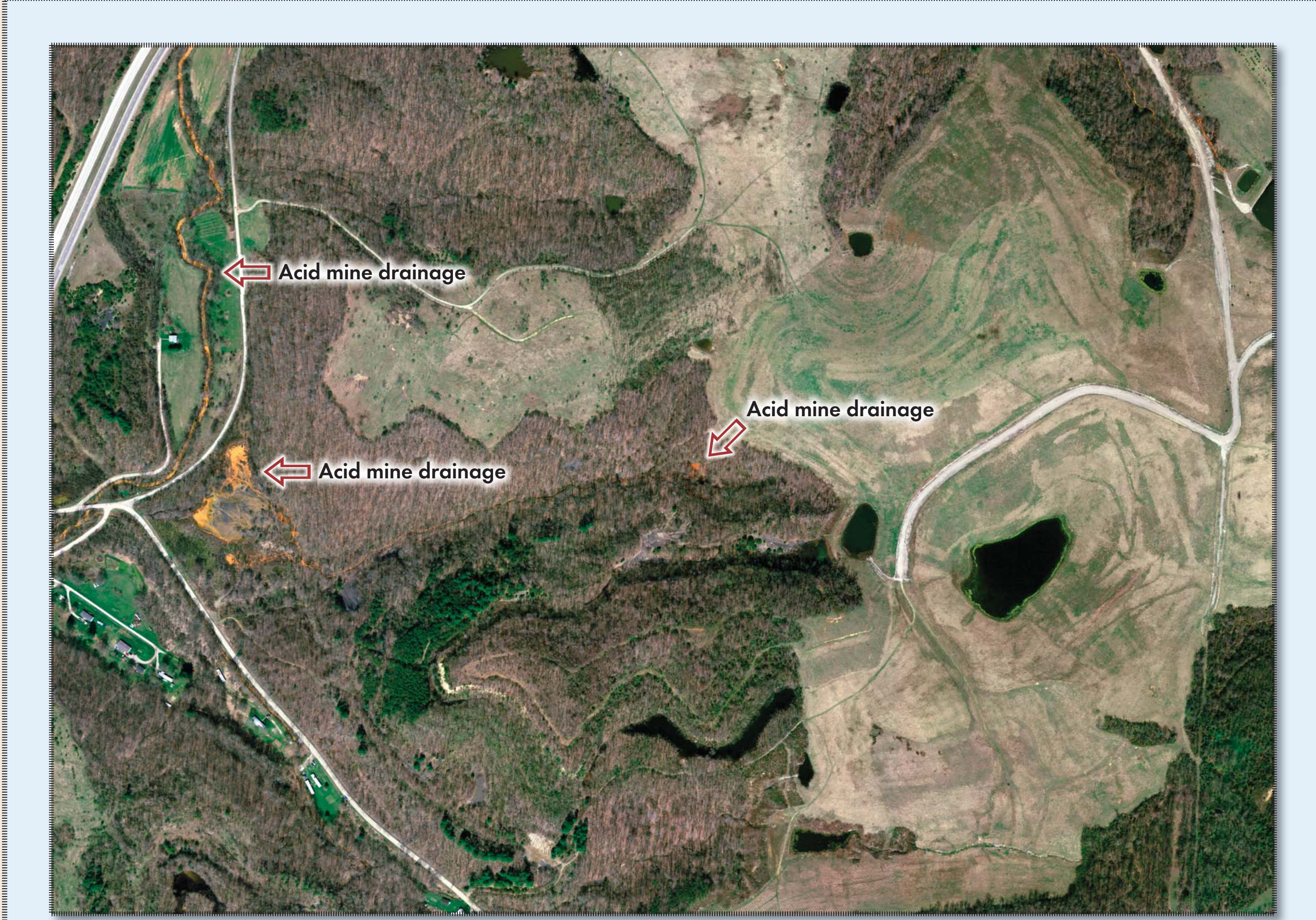
FIGURE 3a.—Locations of abandoned-underground and surface mines near Mulga, Ohio. The orange discoloration is acid mine drainage.
