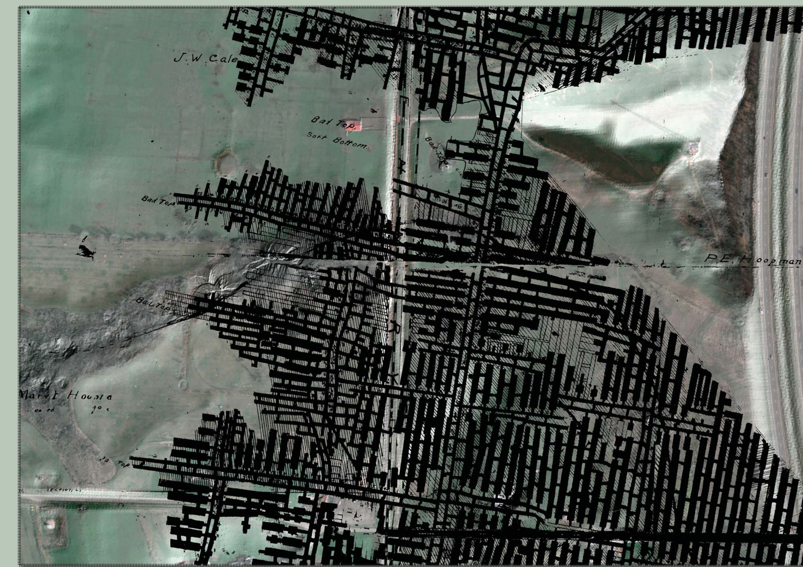
FIGURE 2d.—Overlay of the detailed abandoned mine map. Some of the pit subsidence features lie outside of the mapped mine workings, possibly indicating that the detailed mine map does not completely show the full extent of the mine workings.
