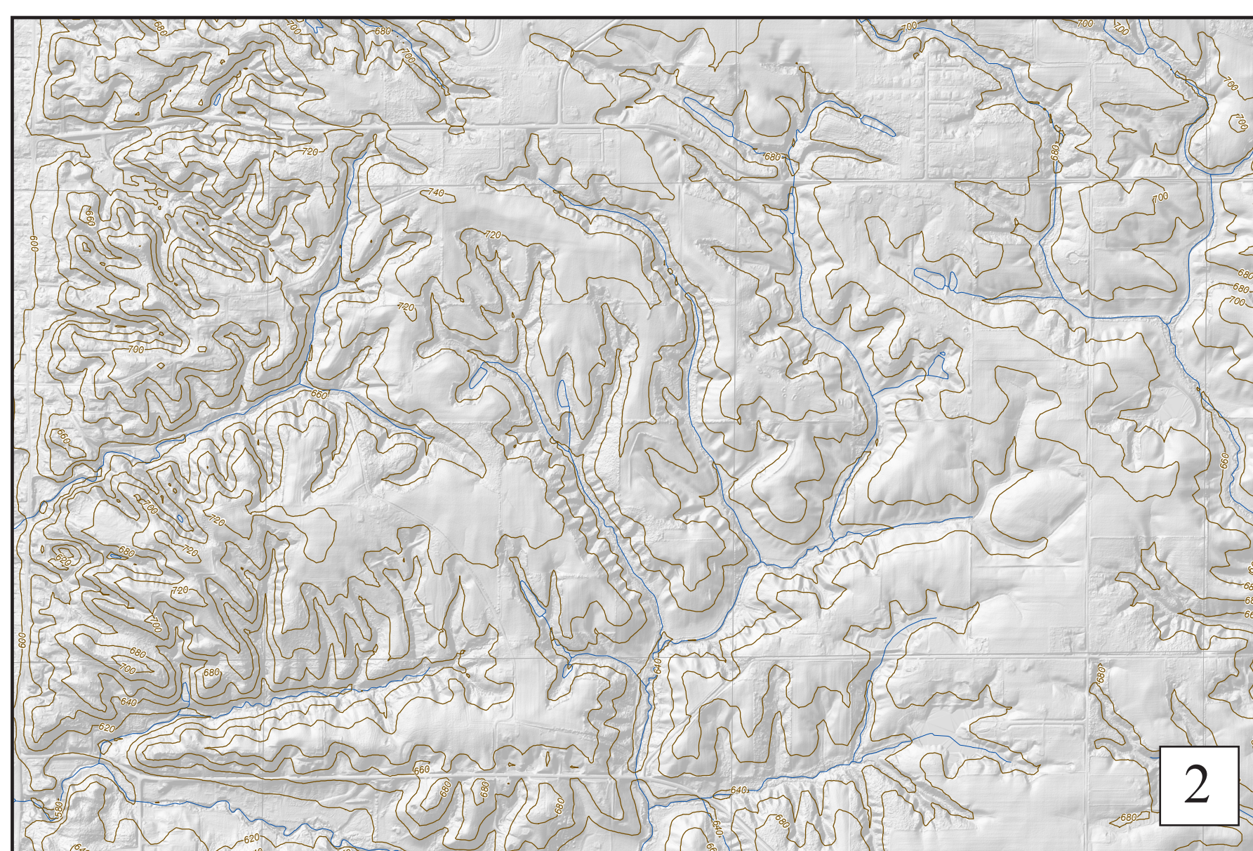
Cartographic contours produced from source 2009 Lidar 1.2 meter resolution DEM data resampled to a one arc-second nominal point spacing (30 meters). The original photogrammetric-based contours in Inset 1 compare favorably to the contours generated from the resampled Lidar DEM. Base image is a shaded relief image produced from the one arc-second Lidar DEM. Despite the significant downsampling of the original Lidar DEM from 1.2 m to 30 m, note the greater landscape feature detail as compared to the one arc-second DEM shown in Inset 1.
