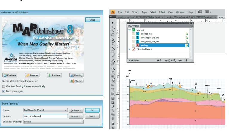
Archived graphics files (.ai, .eps, .pdf)... can be georeferenced to a spatial layer in Illustrator and exported as 2D shapefiles... then converted into 3D shapefiles.
