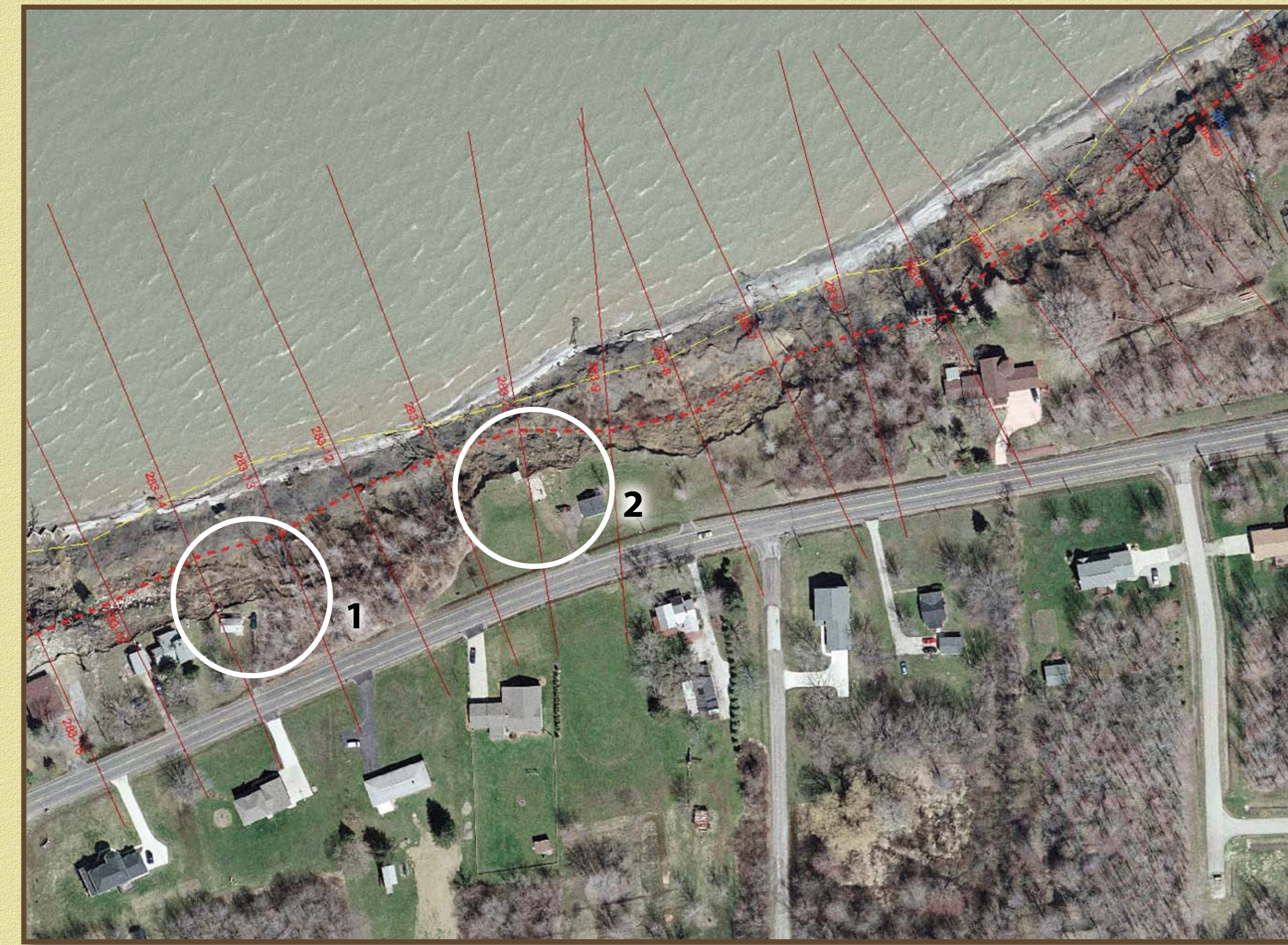
FIGURE 3b.—By 2004, the two houses (circled) have been lost to coastal erosion. Property (2) now has a garage.
