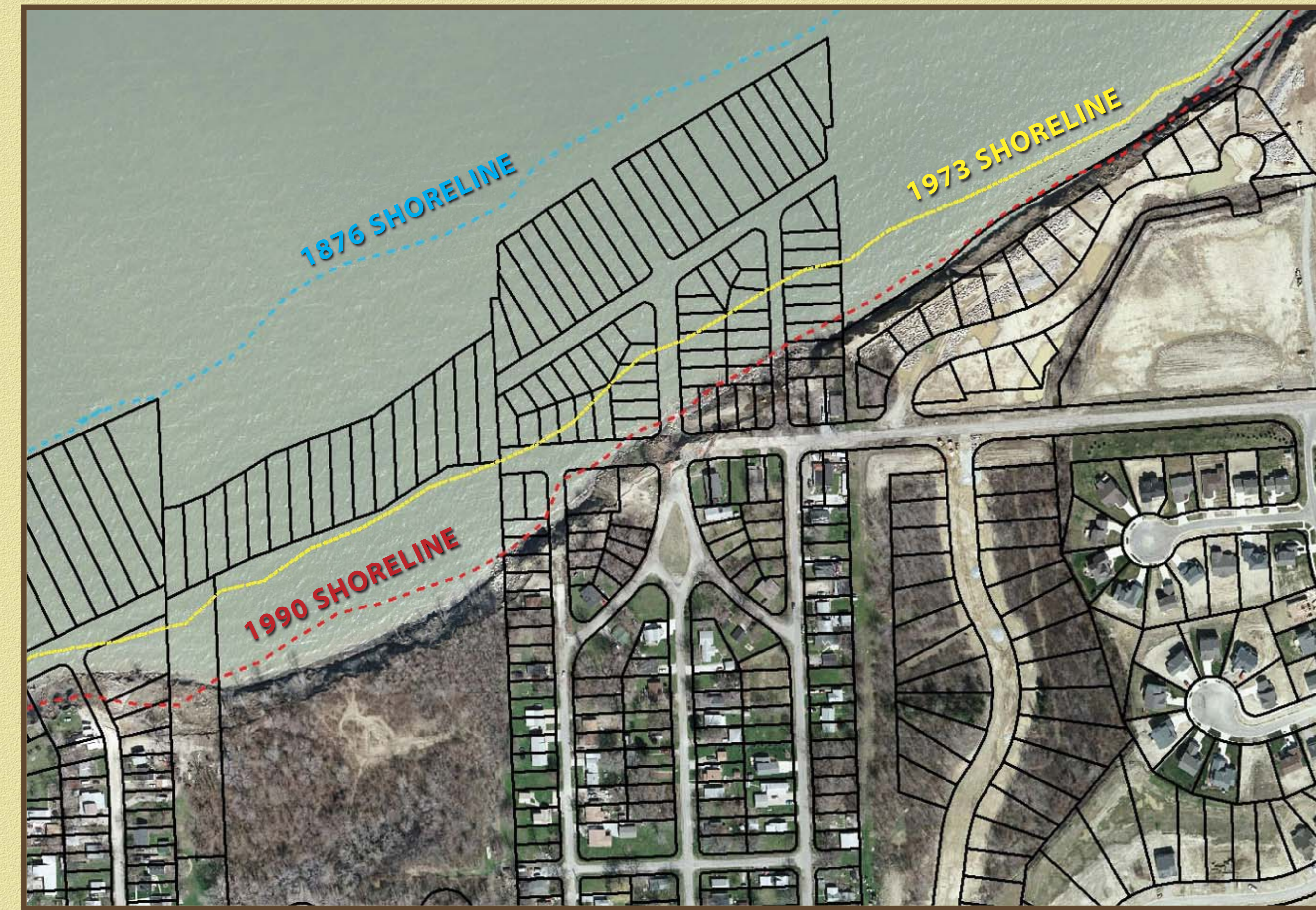
FIGURE 1.—Between 1973 and 1990, Ohio's shoreline receded approximately 24 feet. This area near Painesville experienced up to 207 feet of recession. Numerous parcels (black outlines) have been lost to coastal erosion.
