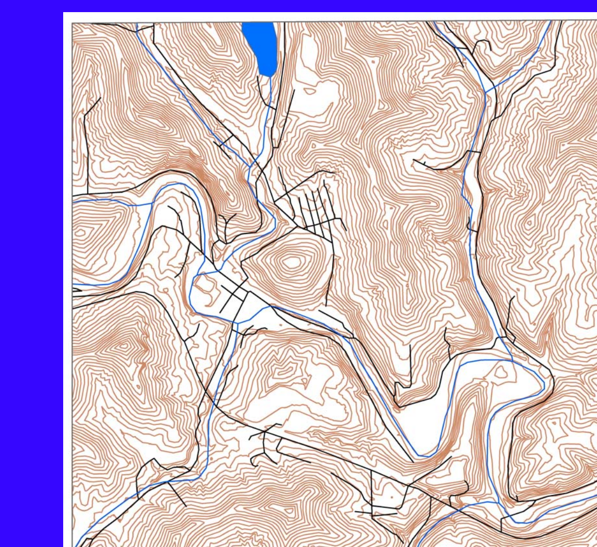
Figure 10. Twenty foot contours and 2006 second edition Census Bureau Tiger Files used for a simple unannotated base map.
