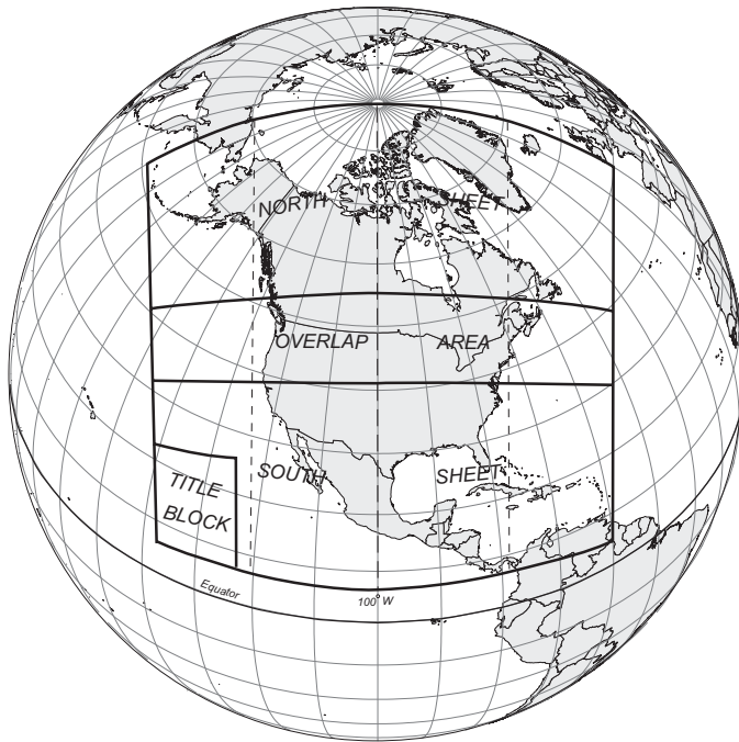
Figure 1. Index map showing the area covered by the Geologic Map of North America. Long-dashed line is the central meridian (100°W); short-dashed lines are small circles where the projection cylinder intersects the sphere and the scale is exactly 1:5,000,000.
