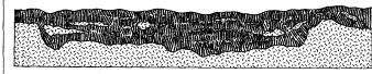
FIG. 2.—Section of a natural exposure of coke and an intrusive sheet on the north side of the Purgatory River opposite Sopris. The structure of the coke is approximately normal to the surface of the intrusive.
