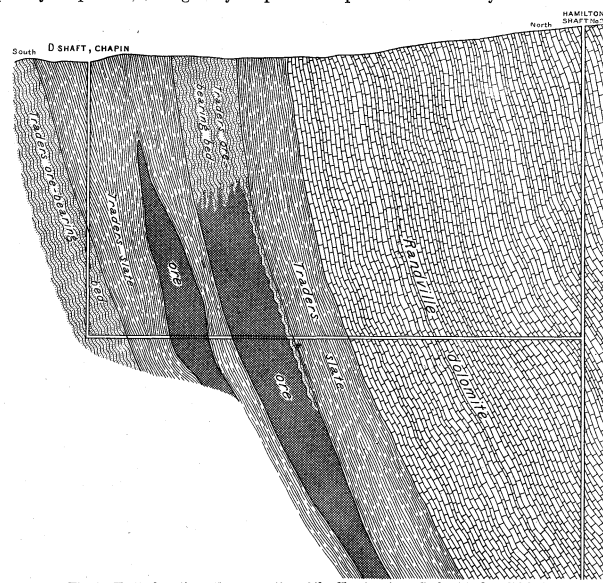
Fig. 4.—Vertical north-south cross section of the Chapin mine. Scale: 1 inch = 250 feet.
