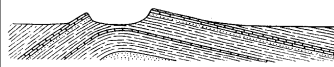
Fig. 13.—The same as a later stage of erosion. The crest of the arch is occupied by a valley in shale. The cut edges of the thicker limestone crown parallel ridges enclosing the valley.
