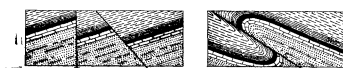
FIGURE 4.—Ideal sections of broken and bent strata, showing (a) normal faults and (b) a thrust or reverse fault.
