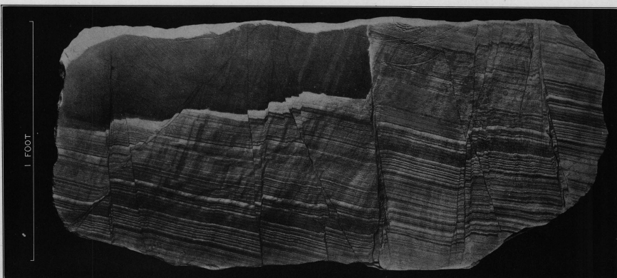
PLATE XXIX.—SAWED BLOCK OF UNKPAPA SANDSTONE FROM LOCALITY WEST OF BUFFALO GAP, SHOWING MINUTE LAMINAE OFFSET BY STEP FAULTS.
