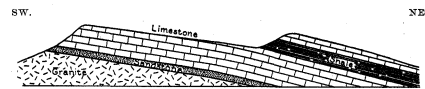
FIGURE 3.—Ideal section across the Silver City Range, illustrating the relation of the asymmetric form of the surface to the geologic structure. Gentle northeast slopes follow the bedding of the rocks; steep southwest slopes cross the edges of the rock layers.
