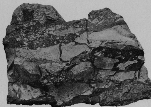
FIGURE 16.—CHERT BRECCIA WITH JASPEROID CEMENT. The angular chert fragments are parts of one mass and are but little displaced.
