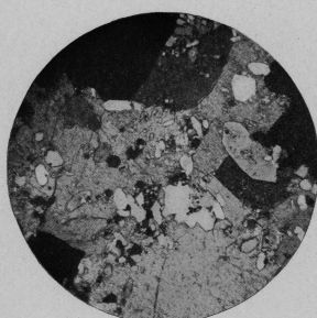
FIGURE 25.—MICROGRAPH OF LIMESTONE BEGINNING TO ALTER TO JASPEROID. Small crystals of quartz are scattered through the limestone.
