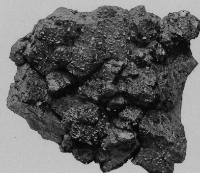
FIGURE 23.—CHALCOPYRITE WITH PARALLEL ORIENTATION ON ZINC BLENDE. From cavity in sheet ground.
