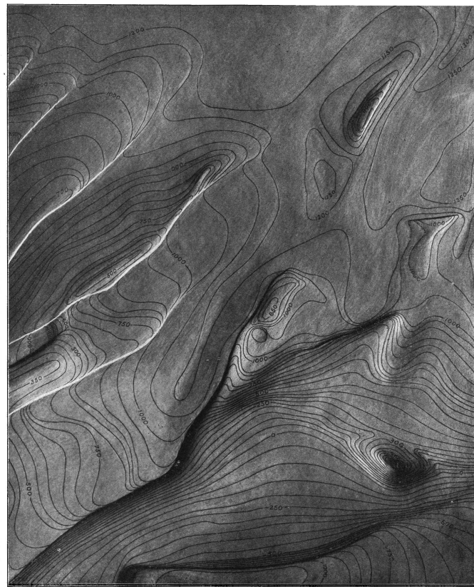
FIG. 2.—Model of the deformed surface of the Boone formation in the Tahlequah quadrangle. The vertical scale is exaggerated to approximately three times the horizontal in order to bring out the smaller undulations. Contour interval is 50 feet. To give the proper impression of the structure the light is made to fall on the surface from the upper left-hand corner.
