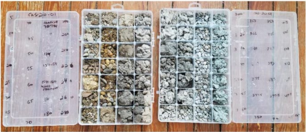
Mud rotary drill cuttings every 5 feet
