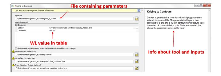
An error report is included to help identify overall error and trouble spots in the raster surface. This report can aid in identifying locations where additional wells can improve the interpolated surface.
