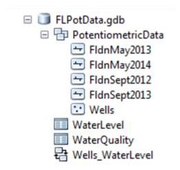
Creating the potentiometric surface contour lines is a two-step process. First, an automated process using kriging is used to make a raster surface of the water-level data. This process is saved and documented in an ArcGIS Toolbox.
