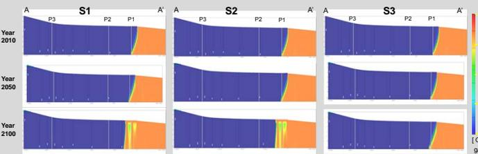
Calculated position of the salt water front in bottom layer for different distances from river (Δy)
