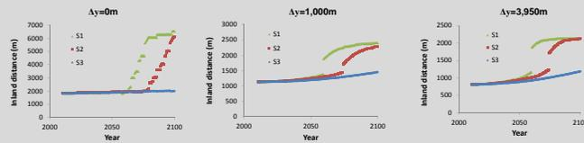
By year 2100, in S1 and S2, the toe of the salt water front migrates 4.6 km in the aquifer under the river. The toe does not migrate significantly in S3 at that location. At 3.95 km from the river, the toe migrates 1.5, 1.5 and 0.5 km for S1, S2, and S3, respectively
