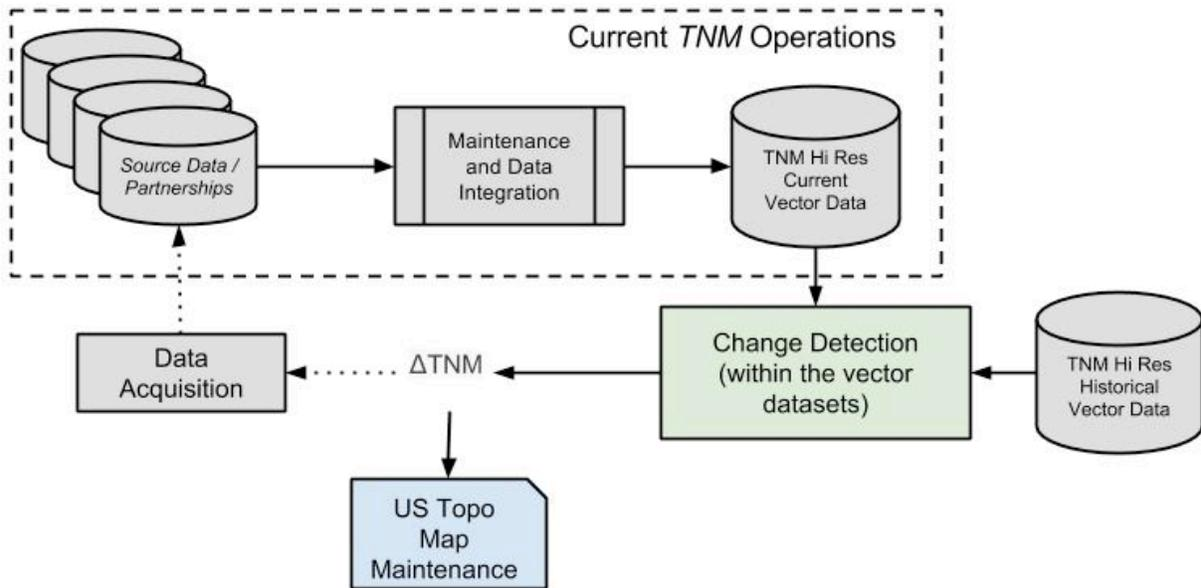
Figure 6. NGTOC Change Detection Proposed Concept of Operations.
