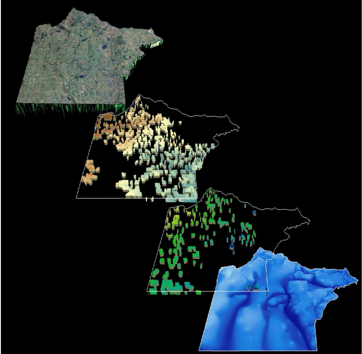
Figure 5. Four grids representing the surface elevation with wells, two (out of 14) stratigraphic sand unit grids and the bedrock elevation grid.
