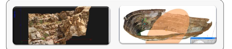
Generates accurate, scaled 3D images of rock faces from stereo photographs taken in open pit, underground and other inaccessible rock faces. Enables structural mapping directly on to 3D surfaces with immediate geotechnical results.
