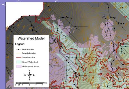
Figure 5. Watershed model of the Sewell coal seam on the Fayetteville 7.5-minute topographic quadrangle and surrounding area.
