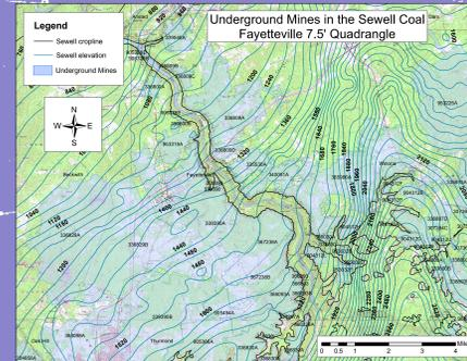
Figure 4. Extent of underground mines in the Sewell coal seam on the Fayetteville 7.5-minute topographic quadrangle and surrounding area.
