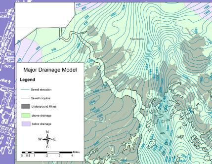
Figure 6. Major Drainage Mining Above/Below Drainage GIS model of the Sewell coal seam on the Fayetteville 7.5-minute topographic quadrangle and surrounding area.
