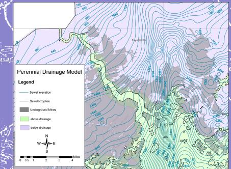
Figure 7. Perennial Drainage Mining Above/Below Drainage GIS model of the Sewell coal seam on the Fayetteville 7.5-minute topographic quadrangle and surrounding area.
