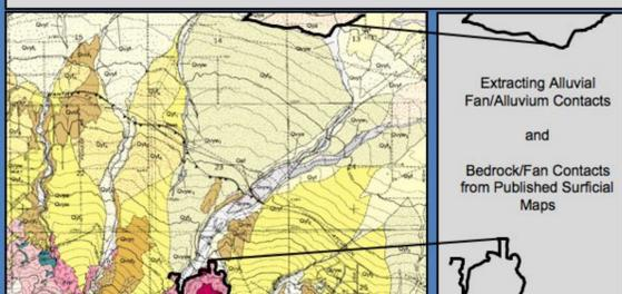
Figure 3: Areas underlain by quaternary sediment that may include aggrading alluvial fan segments subject to alluvial fan flooding are mapped by extracting the bedrock contact with alluvial fan and alluvial wash deposits, providing the contact along the mountain front. The contact between alluvial fan deposits and axial valley deposits are also extracted and then the upper and lower contacts are merged to form polygons that represent all Quaternary age alluvial fan deposits.
