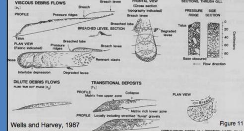
Figure 11: Subsurface profiles of debris flow deposits indicate that they are commonly matrix supported, inversely graded at their base, and normally graded at the top. They are also characterized by a lack of bedding (usually massive) and a lack of clast imbrication.
