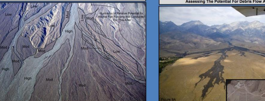
Figure 6: Illustration of a the relative hazard to alluvial fan flooding on an alluvial fan in the Santa Rosa Mountains, Riverside County, CA.
