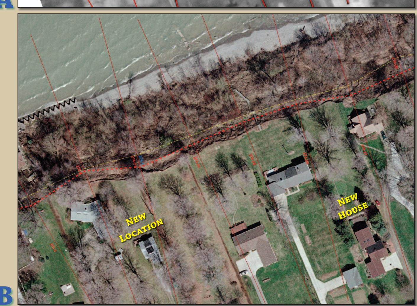
As a bluff recedes, buildings can be destroyed from the erosion, torn down before they are destroyed, or physically moved back from the bluff. Here two houses have disappeared, one of which is a 3,500 square foot house. In addition, a house has been moved back from the bluff edge.
