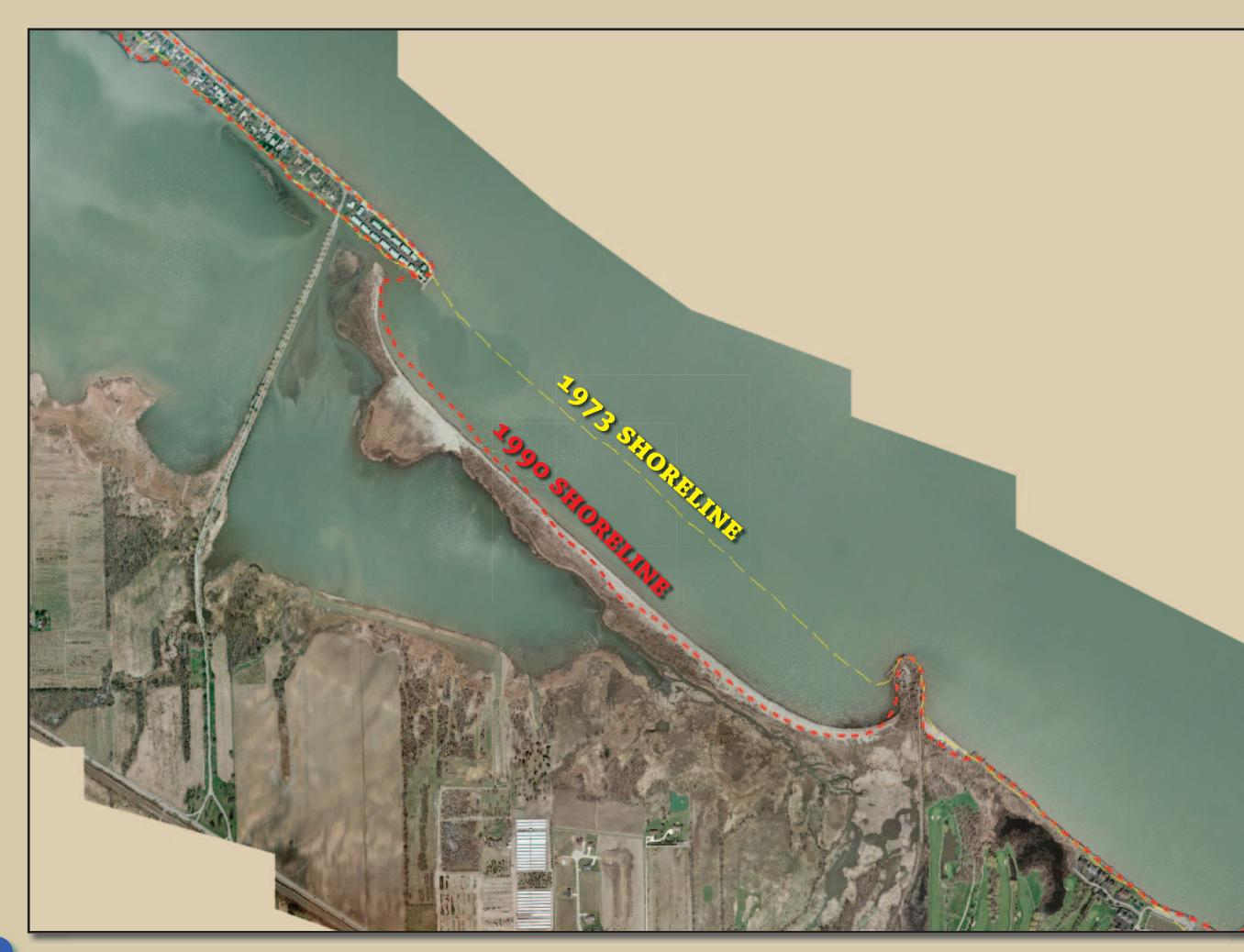
The Lake Erie coastline of Ohio is very dynamic and can undergo large-scale changes. The Sheldon Marsh barrier island, which was blown out during the great November 1972 storm, has been retreating at a rate between 15 to 56 feet per year.
