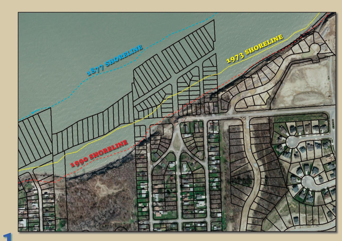
Erosion along the Lake Erie shoreline of Ohio is a major geologic hazard. Between 1973 and 1990, the average shoreline recession was 1.41 feet per year, which indicates that the shoreline receded approximately 24 feet during the 17-year period. This figure shows an area of the coast near Painesville, Ohio, that has undergone up to 207 feet of recession during the 17-year period.
