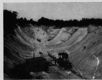
PLATE 27.—CLAY PIT 1 MILE SOUTH OF OREMINIA (MINES) Residual clay accumulated on the outcrop of the Mines dolomite. Looking north.
