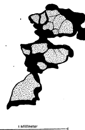
FIGURE 13.—Typical pyrite kernels in chalcocite. Schist ore, 1925 level of the No. 2 mine, Ray district.
