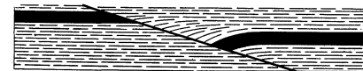
FIGURE 10.—Sketch of normal fault in Willow mine, south of Van Houten. The coal bed, which has been dropped about 15 feet, is bent downward on the downthrown side of the fault, as if it had been subjected to compression and slight upthrusting after the original faulting.
