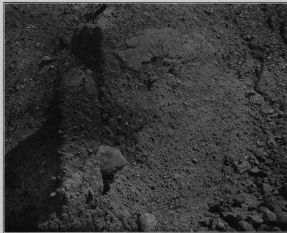
PLATE V.—SECTION OF ILLINOIAN TILL TEMPORARILY EXPOSED IN BED OF DETROIT RIVER NEAR STONY ISLAND DURING EXCAVATION OF LIVINGSTONE CHANNEL. This till is very stony compared with the Wisconsin till, shown in Plate VI.
