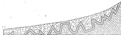
FIGURE 9.—Sketch of the structure at Fluted Rocks, W. Va. The formation shown by the dot pattern is the Keefer sandstone member of the McKenzie formation, which stands in relief, as shown in Plates X, XI, and XIV.
