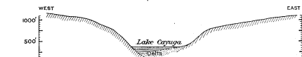
FIGURE 3.—Cross section of Lake Cayuga valley 2 miles north of Ithaca. Horizontal scale, 1 inch=2 miles.
