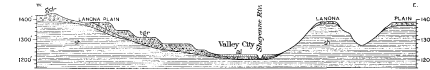
FIGURE 3.—Section across Sheyenne Valley at Valley City. Horizontal scale, 1 inch = 400 feet approximately. Several river terraces are shown below the high Lanona plain: a, Shale; g, glacial drift; t, terrace gravel; al, alluvium.
