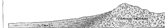
FIG. 13.—Cross section showing the relation of outwash (stratified drift) to the terminal moraine, similar to that which exists southeast of Plainfield.
