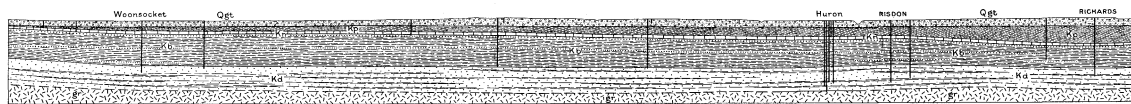
Fig. 1.—Sketch section across the Huron quadrangle along a line through Woonsocket and Huron, showing the artesian wells in the vicinity extending to the Dakota water-bearing sandstone. Qgt, Glacial till; Ks, Pierre shale; Kd, Niobrara formation; Ks, Benton formation; Kd, Dakota formation; g, granite, including probably overlying Sioux quartzite in places. Horizontal scale: 1 inch=3 miles. Vertical scale: 1 inch=100 feet.
