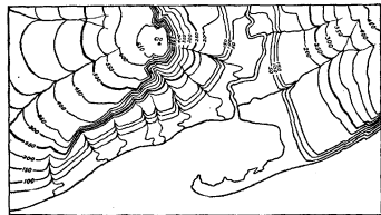
Fig. 1. The upper figure represents a sketch of a river valley, with terraces, and of a high hill circled by a cliff. These features appear in the map beneath, the slopes and forms of the surface being shown by contours.
