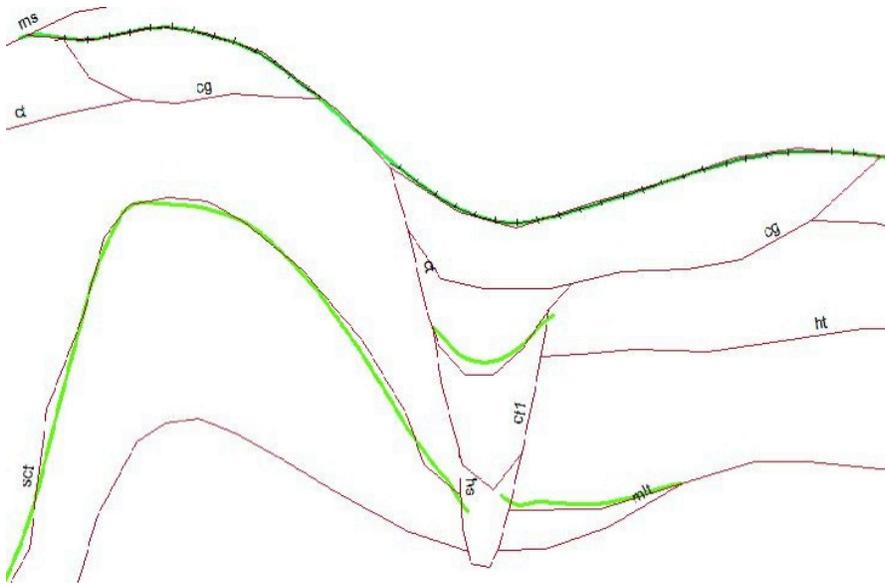
Figure 6. Final grid elevation for a bottom unit (shown in green hatched line) along with the original geologic cross section (shown in red). Profiles of the final grid tops and bottoms of each unit can be checked against the original geologic cross section. This is used to identify any gridding errors and pin point specific locations for making corrections.
