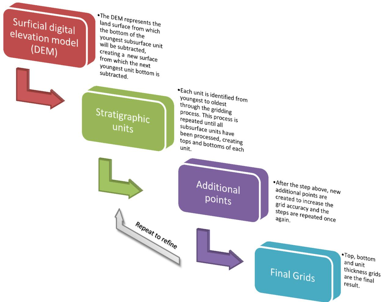
Figure 4---A digital elevation model (DEM) establishes the initial elevation and then the base of each unit is subtracted from the unit above in the sequence from youngest to oldest (i.e. Malolepszy, 2006). This creates the top, bottom and unit thickness grids for each stratigraphic unit.
