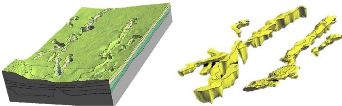
Figure 1. Example of modelling derived three-dimensional depiction of sand bodies with a complex geometry, resulting from deposition in a glaciated landscape. Subsurface extent of sand body is shown in right-hand figure.
