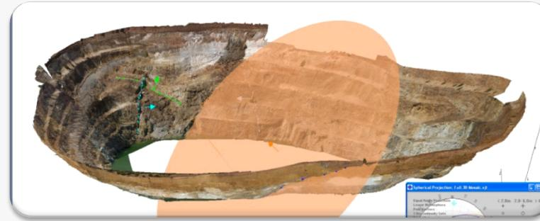
Generates accurate, scaled 3D images of rock faces from stereo photographs taken in open pit, underground and other inaccessible rock faces.
