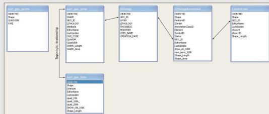
FIGURE 2.—Entity-Relationship diagram for the three-dimensional surficial geology dataset. Note that the surficial-geology polygons have a 1-to-many relationship with the lithology table. Each polygon, while only displaying the unit at the surface, is actually associated with multiple lithologic units from the surface to the bedrock.
