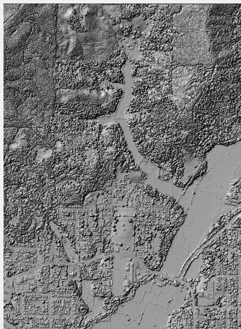
The highest hit elevation model is a representation of the full-featured landscape at the time of the lidar aerial survey. As opposed to the last-return (ground) illustrated by the bare earth elevation model, the highest hit is the first-return to the lidar sensor -- be it tree, car, sky-scraper, or even people. Though not as immediately useful for applications in geology as the bare earth elevation model, it has many merits when it comes to feature extraction for base mapping.
